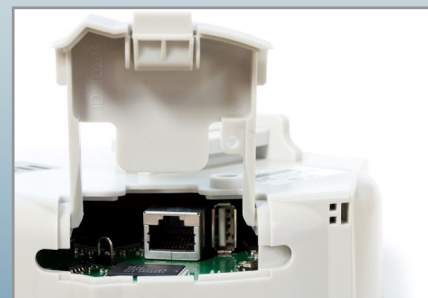
Easy to access enclosure, door latches open
